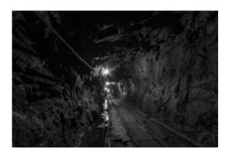
Three workers were crushed by a rockfall in a mine tunnel, resulting in one death. The fatality occurred when the experienced mine crew was working near the site of a previous incident caused by a rockfall. There was a large crack in the rock. Concern about partial collapse of the sides of the tunnel resulted in a meeting between the foreman and a rock specialist. They had noted a smaller crack was forming a wedge-shaped rock which could fall.
