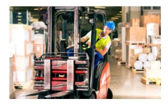
Powered industrial trucks, commonly called forklifts or lift trucks, are used in many industries, primarily to move materials. They can also be used to raise, lower, or remove large objects or a number of smaller objects on pallets or in boxes, crates, or other containers. Powered industrial trucks can either be ridden by the operator or controlled by a walking operator.
