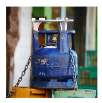
A small business owner had been using an oxy-acetylene cutting torch. In an effort to save money on rental charges for the oxygen cylinder, he was attempting to transfer the remaining oxygen into a propane cylinder. The cylinder was supposedly empty, but actually contained propane. He had rigged up a hose system linking the two cylinders. As soon as he cracked the oxygen valve open and began the transfer, an explosion occurred and he was killed.
