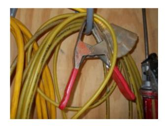
A makeshift switch on a sandblasting unit apparently set off an explosion of gasoline vapors killing a worker who was cleaning a petroleum storage tank.
