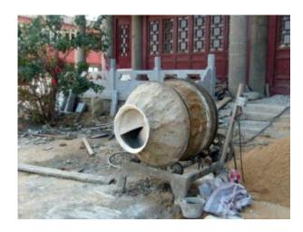
An 18-year-old laborer died after becoming entangled in a portable mortar mixer.
