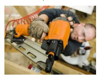
**3. Single Sequence Triggers** which like full sequential triggers, will only fire when the controls are activated in a certain order. First, the safety contact tip must be pushed into the work piece. Then, you must squeeze the trigger. To fire a second nail, you only need to release the trigger.
