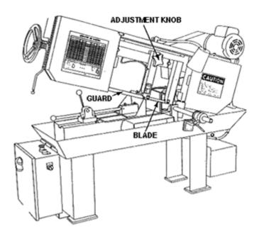
3. Interlocked guards that automatically shut off or stop the machine when a tripping
