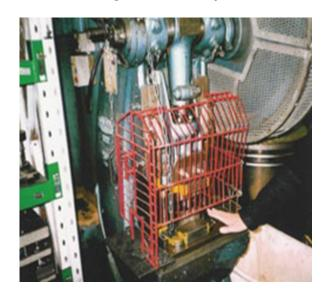
**The good news** is that the mechanical power press in this picture has a frontal machine guard to prevent workers from reaching into the point of operation, i.e., the place on the machine where the material is placed so it can be cut, stamped, sheared, etc.
