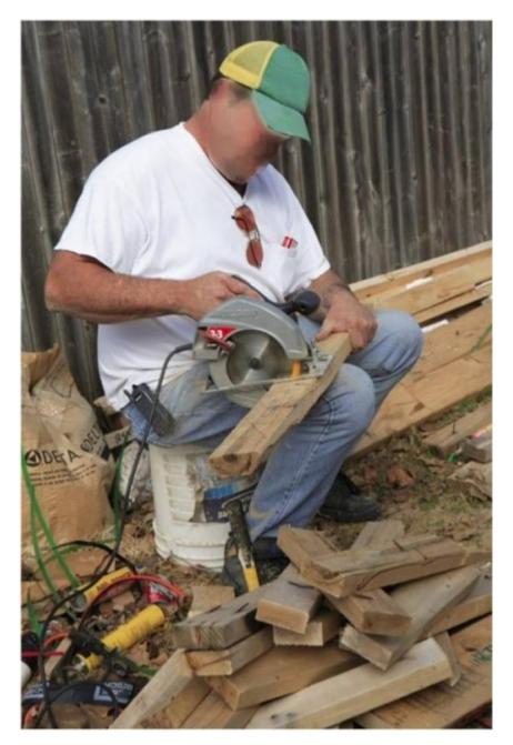
Of all the dangerous things the worker operating this handheld circular saw is doing, the one that scares me the most is using his legs to brace the board he's cutting.
