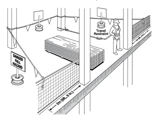
When reinstalling or rebuilding a guardrail, make sure it is installed as intended according to the manufacturer's instructions or its original design. Store the removed guardrails or sections in a place where they cannot fall on someone or become a trip hazard.
