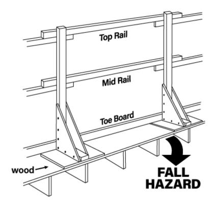
Regardless of type, make sure all guardrails used meet the regulatory requirements and are built according to requirements (e.g., height and spacing requirements of guardrail components and/or are installed according to the manufacturer's instructions.
