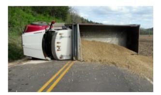
Overturn of the bed of the truck or the entire truck it self is one of the major hazards for the operation of the truck. Trucks vary greatly in design. But the basic premise of the job they complete is universal. That is, dump trucks haul material and dump the material. Regardless of varying designs and uses of the trucks, many of the hazards of operation remain the same.
